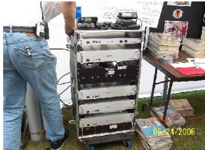
W4OZK, Greg and KA4KUN, Jay set up a demonstration of the Icom® D-Star® at our Field Day site on Saturday afternoon. This is the basic setup for a repeater. It contains a 2 meter, 440 mHz, and a 1.2 GHz digital repeater system. A portable tower mounted on a trailer, which could be extended, was also demonstrated as part of a movable system that could be set up anywhere it might be needed for emergency communications. Internet capability was also included with a Starband® satellite system.
